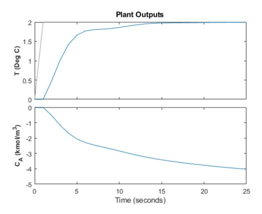
The plant/model mismatch degrades controller performance slightly. Degradation can be severe and must be tested on a case-by-case basis.
