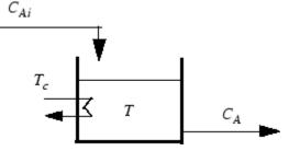
Measurement of reactant concentrations is often difficult, if not impossible. Let us assume that T is a measured output,  $C_A$  is an unmeasured output,  $T_c$  is a manipulated variable, and  $C_{Ai}$  is an unmeasured disturbance.
