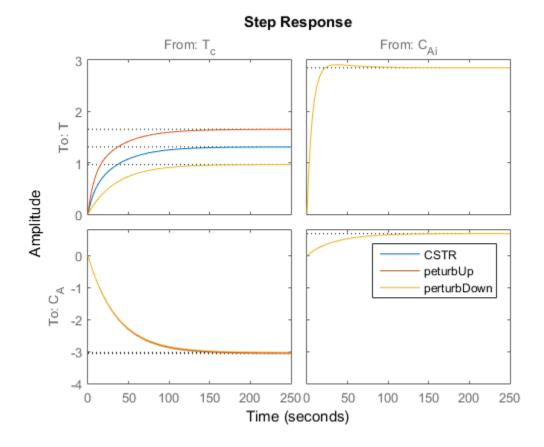
Perturbing element B(2,1) of the CSTR plant changes the magnitude of the response of the reactor temperature, T, to changes in the coolant temperature, Tc.
