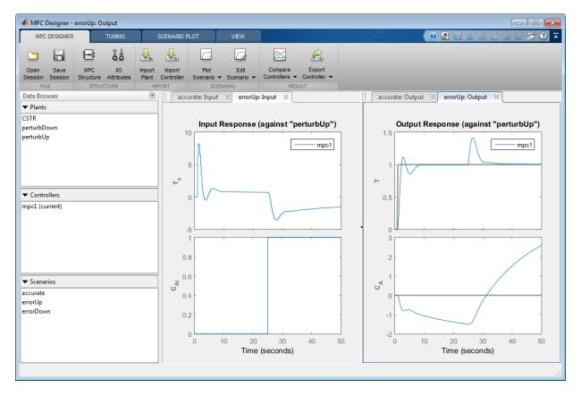
The app creates the **errorUp: Input** and **errorUp: Output** tabs, and displays the simulation response.
