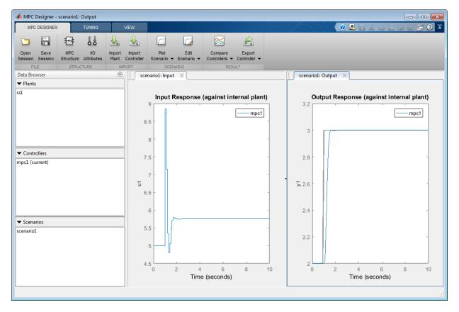
The default controller tracks the output reference value well, however the initial controller response is aggressive.
