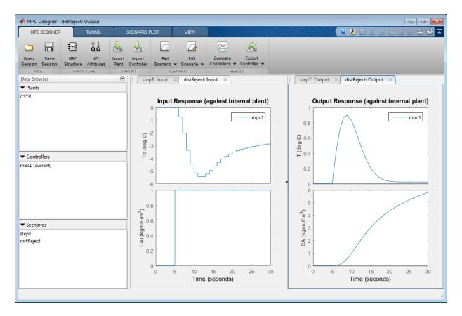
In the **Output Response** plots, the controller returns the reactor temperature, **T**, to a value near its setpoint as expected. However, the required control actions cause an increase in the output concentration, **CA** to  $6 \text{ kgmol/m}^3$ .
