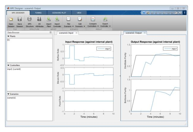
When launched with a continuous-time plant model, such as DC, the default controller sample time is 1 in the time units of the plant. If the plant is discrete time, the controller sample time is the same as the plant sample time.
