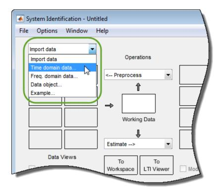
In the Import Data dialog box, specify the **Input**, **Output**, and **Sample time** using the data from the MATLAB workspace.
