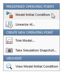
The model initial condition is the default operating point for linearization in **MPC Designer**.
