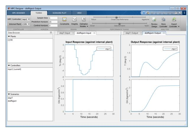
In the **Output Response** plots, once the reactor concentration, **CA**, approaches 3 kgmol/m<sup>3</sup>, the reactor temperature, **T**, starts to increase. Since there is only one manipulated variable, the controller makes a compromise between the two competing control objectives: Temperature control and constraint satisfaction. A softer output constraint enables the controller to sacrifice the constraint requirement more to achieve improved temperature tracking.
