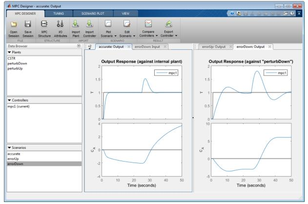
The perturbation creates a plant, perturbDown, that responds slower to manipulated variable changes than the controller predicts. On the **errorDown: Output** tab, in the **Output Response** plot, the setpoint tracking and disturbance rejection are worse than for the unperturbed plant.
