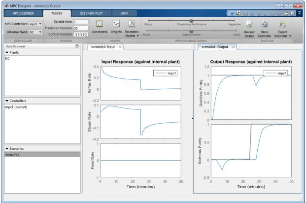
The initial manipulated variable moves are much smaller and the moves are less oscillatory. The trade-off is a slower output response, with larger interactions between the outputs.
