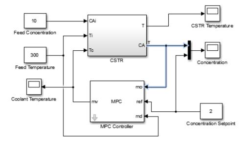
The CA signal can now be used to define output specifications for calculating a model steady-state operating point.
