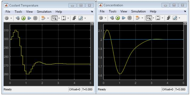
The **Concentration** output response is similar to the **UD\_reject** response, however the settling time is around 1 second later. The different result is due to the mismatch between the linear plant used in the **MPC Designer** simulation and the nonlinear plant in the Simulink model.
