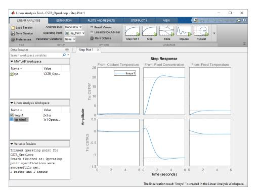
The step response from feed concentration to output CSTR/2 displays an interesting inverse response. An examination of the linear model shows that CSTR/2 is the residual CSTR concentration, C\_A. When the feed concentration increases, C\_A increases initially because more reactant is entering, which increases the reaction rate. This rate increase results in a higher reactor temperature (output CSTR/1), which further increases the reaction rate and C\_A decreases dramatically.
