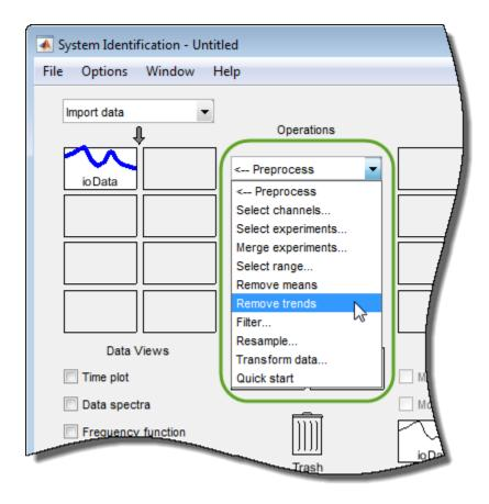
The app creates a data object, ioDatad, using the preprocessed data, and adds this object to the **Data Views** area.
