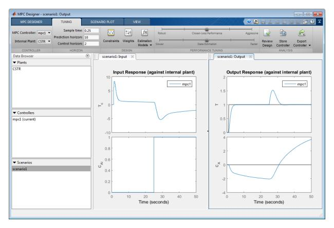
The app runs the simulation scenario, and updates the response plots to reflect the new simulation settings. For this scenario, the internal model of the controller is used in the simulation. Therefore, the simulation results represent the controller performance when there are no prediction errors.
