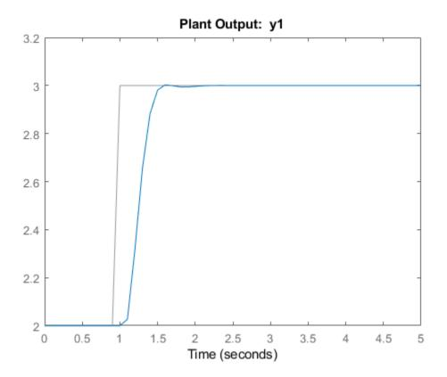
The default controller tracks the output reference value well, however the initial controller response is aggressive.
