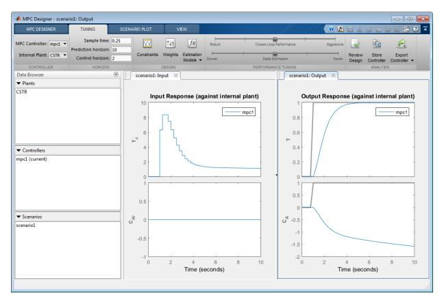
The **Input Response** and **Output Response** plots update to reflect the new sample time.
