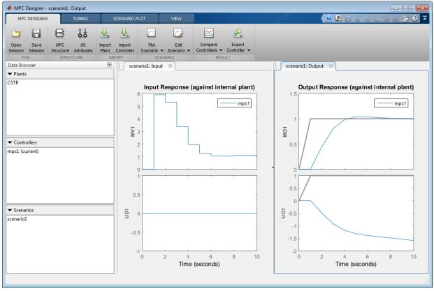
Tip To view the response plots side-by-side, on the View tab, in the Tiles section, click Left/Right.
